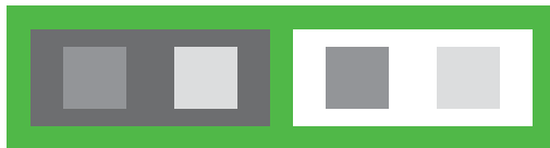
Fig 2: perception of the levels of vs background contrast: the difference in hue appears greater on the white background.
